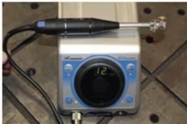
POWER CHECKERING TOOL FIXTURE BY HOSFORD AND CO. WITH AN NSK POWER SOURCE. HOSFORD AND CO. IS ONE OF THE FEW POWER CHECKERING TOOL MAKERS IN PRODUCTION
